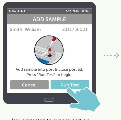
User prompted to expose port on cartridge, add sample, and run test
