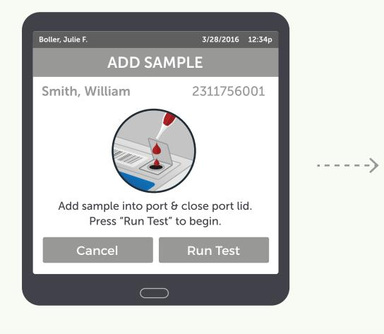
User prompted to expose port on cartridge, add sample, and run test
